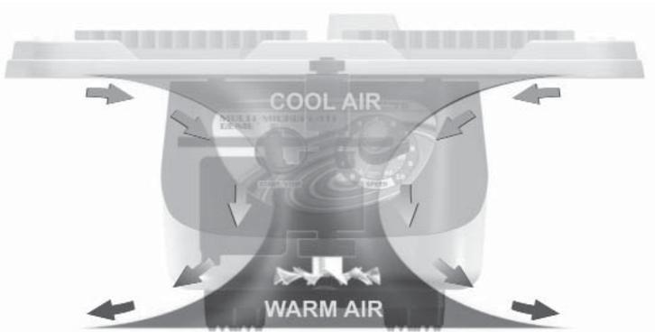
**Heat will not be transferred to your microplates.** The fan (located in the bottom of the unit) directs air downward and out of the unit. As a result, room air is constantly drawn into the unit underneath the tray that holds the microplates, insuring that samples will not be heated.
