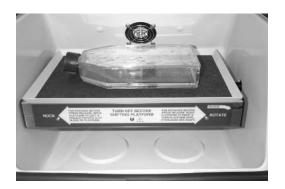
To rotate or rock bags, select mode of operation (Rotate or Rock); locate the bags in the desired position using 2 or 4 (depending on application) magnetic stainless steel mounting strips to hold them in place. Four mounting strips are supplied – more can be ordered (see Accessories). The platform capacity for bags can also be expanded (see Accessories).
