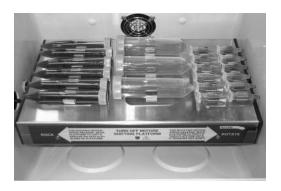
Positioning the plates as shown below will produce a combination rotating/rolling motion ("Figure 8" motion) in the tubes. Adjust the angle to achieve the desired motion.
