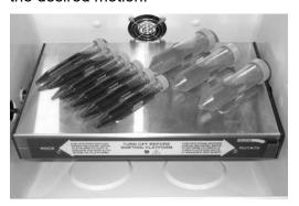
NOTE: When rotating tubes, rotate the magnetic platform by hand before starting, to check the clearance of the tubes to the chamber walls.
