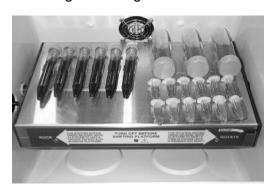
Positioning the plates as shown below will produce a rolling or rocking motion in the tubes.
