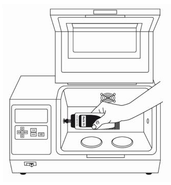
If you don't have a tachometer available, install the magnetic platform and use a stopwatch to accurately measure 360° rotations of the platform per minute. Use masking tape to mark a reference point on the front side of the platform and a connecting point on the incubator wall. This will assist in keeping track of the tray rotations.
