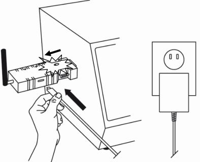
Make sure your PC is connected to the internet and allows drivers to be installed automatically. Plug in the Bluetooth dongle supplied with the wireless adapter to an available USB slot in your PC. Windows will begin automatic installation of device driver software.
