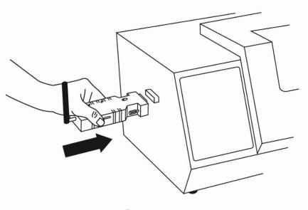
Plug in the power supply cable to adapter socket marked "5VDC", and verify that slide switch on the adapter is in the "SEND" position, pointing towards the antenna connector.
