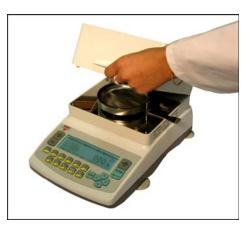
2. Using the Pan Handle, place the Disposable Pan on the Pan Support.
