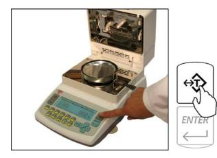
4. Place the sample on the Disposable Pan. After the Tare has been performed, the Disposable Pan can be removed from the Pan Support by using the Pan Handle to evenly distribute the sample.
