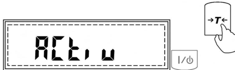
3. All main menu functions and commands will begin to scroll. Enabled functions will have the symbol "o" displayed in the lower left corner of the display.
