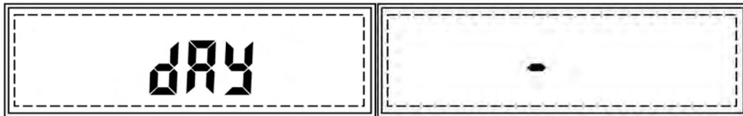
8. Use the following keys to enter the current day setting: the C key to increment a digit, the T key to accept and go to the next digit, and MENU to accept the day setting.
