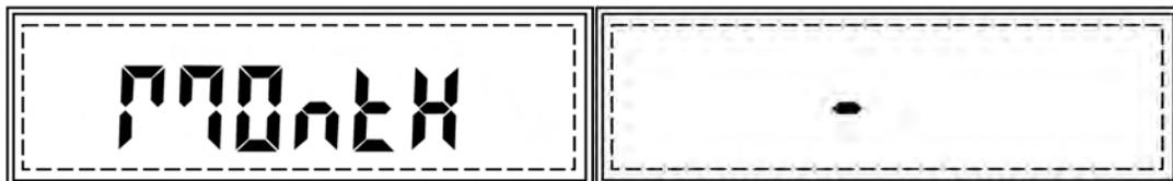
6. Use the following keys to enter the current month setting: the C key to increment a digit, the T key to accept and go to the next digit, and MENU to accept the month setting.
