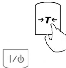
5. Commands "ON" and "OFF" will begin to scroll sequentially. To deactivate the function from the main menu, press the T key when "OFF" is displayed. To activate the function for the main menu, press the T key when "ON" is displayed.
