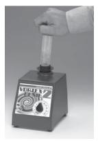
switch into the OFF position. In this mode, you may use any of the accessory attachments available for the VORTEX-GENIE<sup>®</sup> 2 Mixer. *Review instruction No. 3.0 before attempting to change attachments.*
